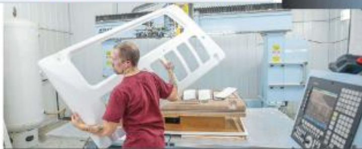
SAY Plastics' James Young lifts a completed air-conditioning unit cover before sending it to a router for cutting and trimming. Mastercam Router software helps machine such large parts despite machine-size limitations.
