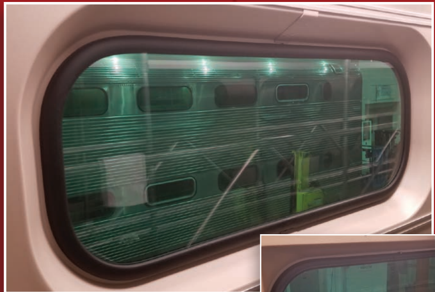
AFTER: New Passenger Rail Thermoplastic Window Mask produced from a polycarbonate blend material with an anti-graffiti cap
