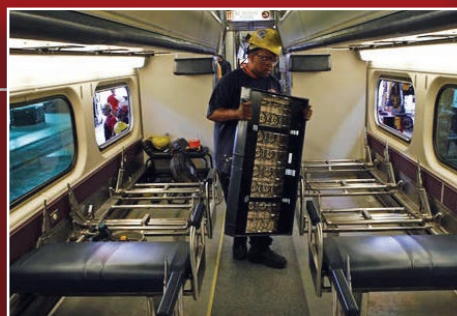
BEFORE: Old Passenger Rail FRP Window Mask beyond service life
