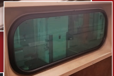
BEFORE: Old Passenger Rail FRP Window Mask beyond service life
