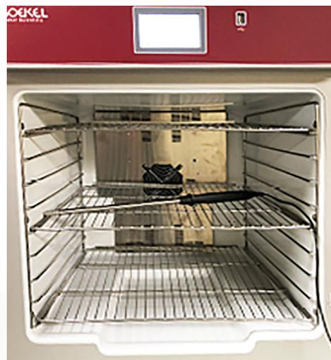
Figure 4: Incubator assembly with deep draw thermoformed liner
