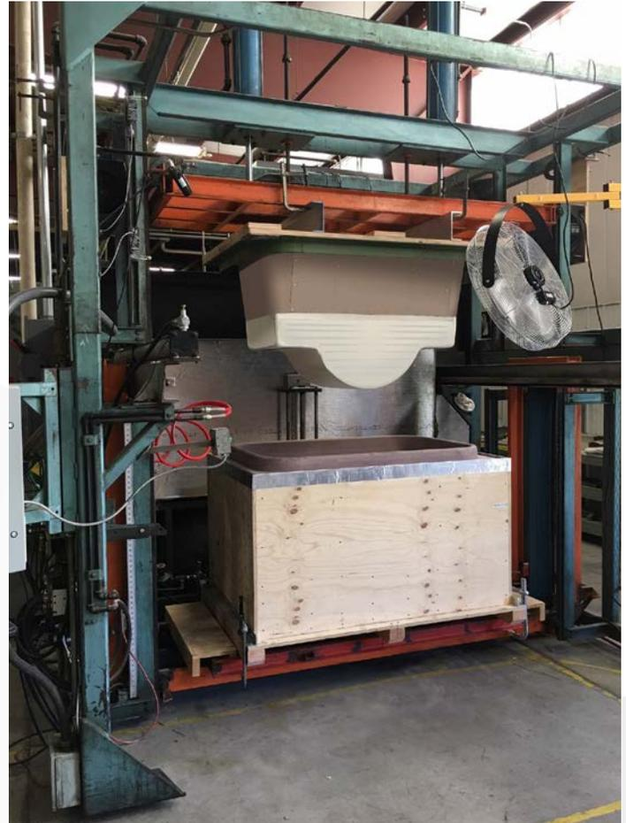
*SAYtooling Mold & Plug Assist setup in deep draw forming machine.*
